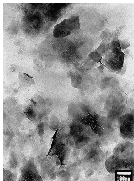
Fig. 2 TEM image of the as-prepared \alpha -cobalt hydroxide.
